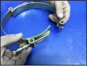
Clamp should be placed on <u>first</u> and <u>second</u> lines on coupler surface.
