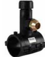
EF TAPPING TEE WITH BRASS OUTLET / EF SERVİS TE DİŞLİ ÇIKIŞLI SDR 11 PE100 WATER / SU : 16 BAR
